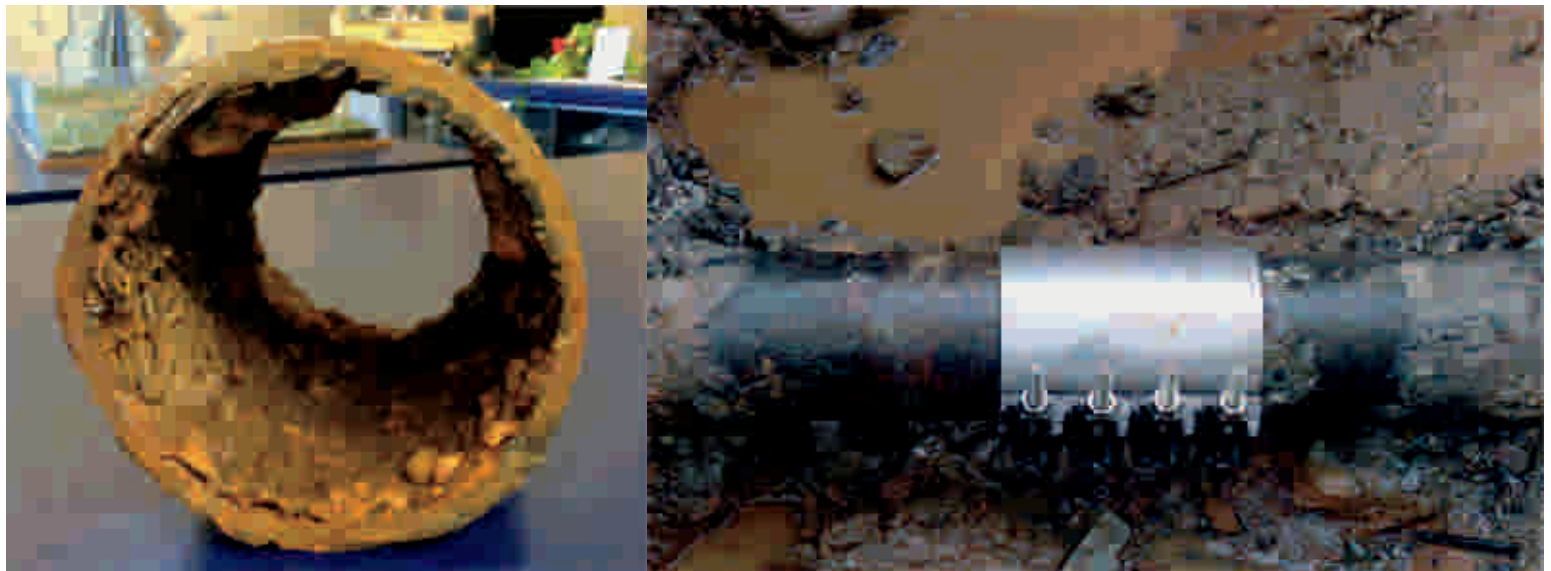
80-year-old cast-iron water main pipe – South Washington Street, Sonora. Repair shown at right.
