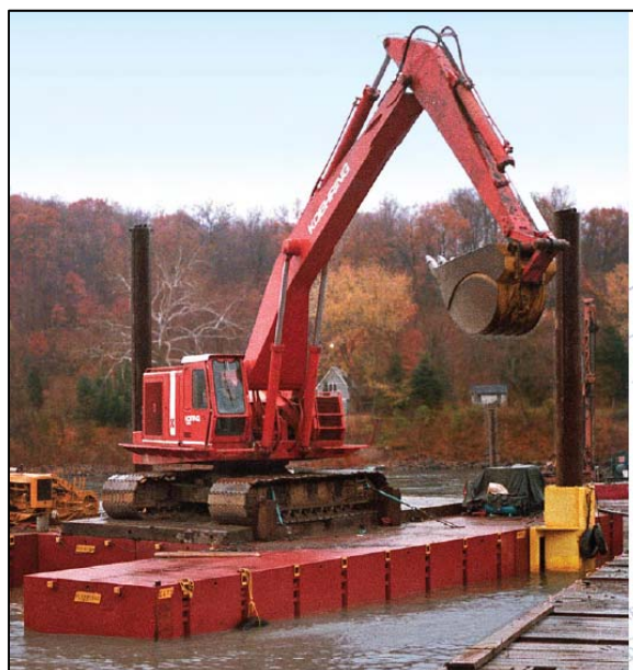
Photo 3.1-13. A modular barge provides a platform for excavation equipment (courtesy of flexifloat.com).
