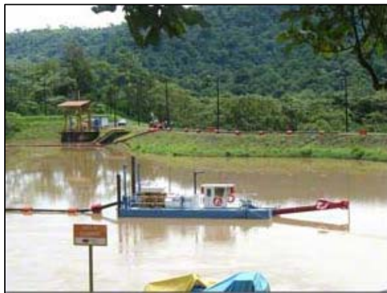
Photo 3.1-12. Example of a small, low draft suction dredge.
